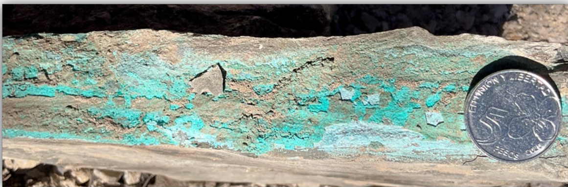
Plate 1: Outcropping, shale-hosted copper oxide mineralization grading 2.4% copper, Mirador project.
