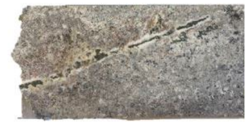
ORG10-08: 131.8m 0.25 g/t Au Granodiorite subvolcanic cut by minor pyrite stringers with white k-spar alteration halos.
