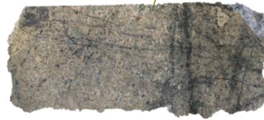
ORG10-05: 208.4m 0.06 g/t Au, 0.9 g/t Ag Dacite porphyry cut by stockwork of grey qtz-py veinlets. Sericite altered.
