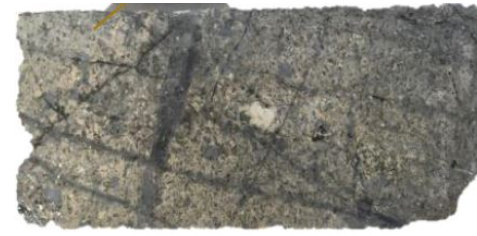
ORG10-06: 140.5m 0.08 g/t Au, 102 g/t Ag Dacite porphyry cut by stockwork of grey qtz-py veinlets. Sericite altered.
