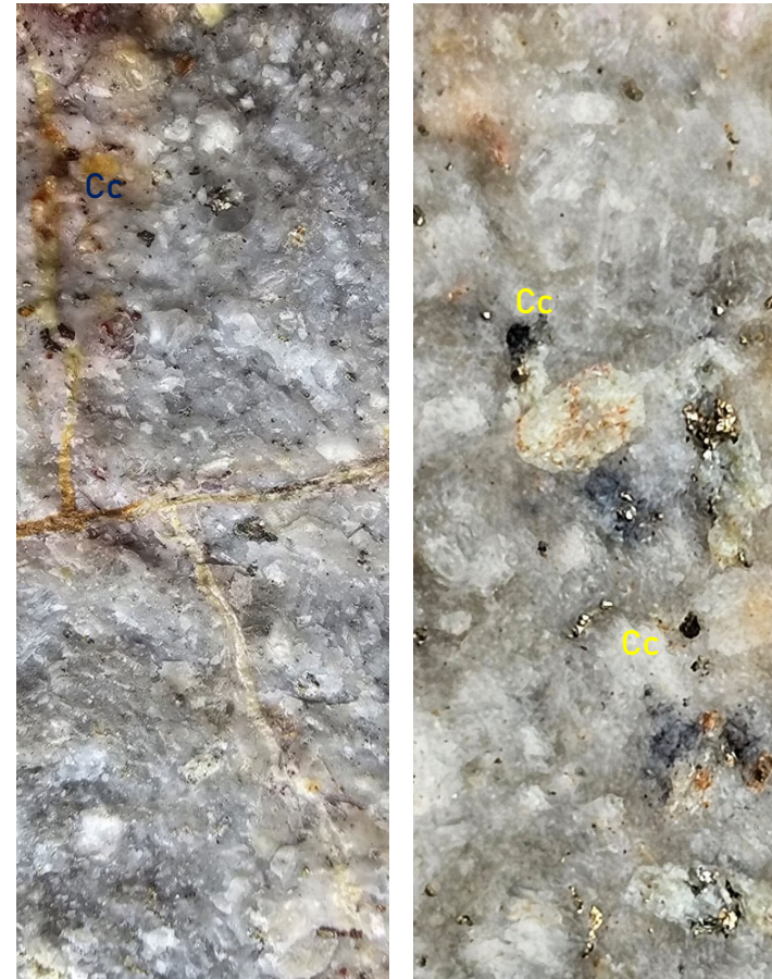
Secondary Mineralization Chalcolite replacing Chalcopyrite in porphyritic rocks
